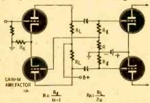
Fig. I-A modern paraphase phase inverter.
