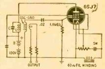
About 1 voit at 60 cycles is taken from the fila-ment transformer and applied to the cathode to vary grid bias. Due to the non-linear tube characteristic the gain varies at 60 cycles and at various harmonics and sub-harmonics of 60 cycles. The 20-cycle sub-harmonic is especially strong because the grid circuit encourages this frequency.
