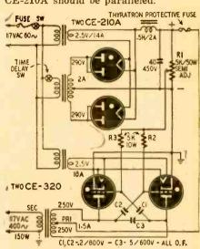
The output frequency depends on the values of R2, R3, C1, C2, and the setting of R1. The value of C3 may have to be changed from that shown.
