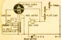
Fig. 5-Working principle of dynamic tester.
