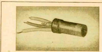
This photo of the mechanoelectronic pickup tube is larger than life.
