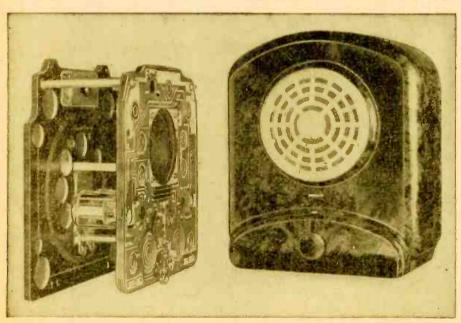
Wiring of this British receiver is appliqued. Molded plastic blanks are sprayed with metal.
