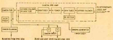
Fig. I—Blanking and sync voltages are usually generated at the master control.
