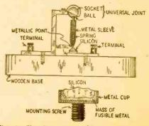
"At first it was a case of trial and er- Fig. 3-The first patented mineral detector.
