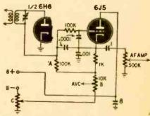
When a signal is received, diode current flows through the i.f. transformer and load to ground. The load is composed of A. B., and part of C. After filtering, only the a.f. component appears at the triode grid. This tube is used as a cathode follower. The circuits of both tubes are common, resulting in regeneration.
