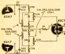
A. This circuit provides high- and lowfrequency equalization. The control networks are in the grid circuits of the 6SC7. They are controlled with dual potentiometers.
