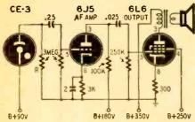
Fig. 2-Amplifier for sound-on-film movies.
