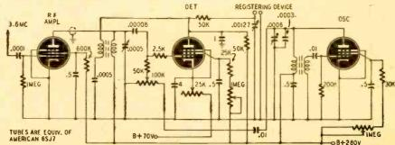
Fig. I—A separately-quenched superregenerator used in the ionospheric experiments.
