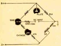
Fig. 2—Fundamental circuit of the voltmeter.
