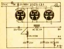
Fig. 5—This eliminator uses vacuum tubes.
