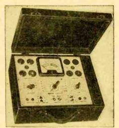
Courtesy Superior Instruments Co. Fig. 2—Standard emission-type tube checker.
