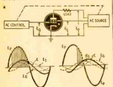
screen-grid is supplied by a voltage (Es) which is 90 degrees out of phase with the plate voltage (Ep). This fixed phase difference may be obtained by using an R-C network within the a.c. source. The control grid voltage (Eg) is variable and in phase with the plate voltage.
