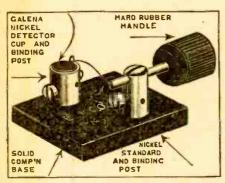
Fig. 4 E. I. Co. crystal detector, designed by H. Gernsback in 1912, orginally sold for 10c for the complete detector. Probably the most widely sold detector at any time. Over 250,000 of these detectors were sold.
