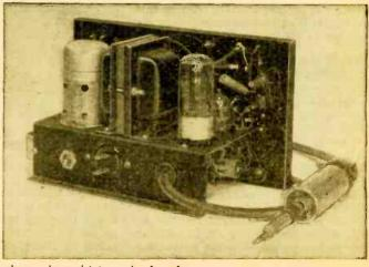
Bottom and rear-chassis views. Isolating condenser is shown plugged into probe for r.f. measurement.
