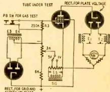
Fig. 3-Fundamental circuit of gm checker.
