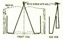
moved. A small loop is made in the wire just under the hook, and a woodscrew and washer serve to fasten the loop to the wall. The remainder of the hanger is bent as shown in the drawing.
