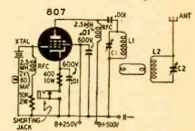
Fig. I-Try a ground at the low end on L2.
