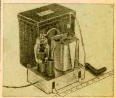
The 25-kilovolt radio-frequency power supply.
