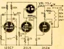
low oscillation frequency—about 1 cycle per second. The output is differentiated by the network R and C, and sharp pulses amplified by the 35L6 are developed across the output choke. A neon lamp, or in this case an OA3/VR-75 tube connected across the choke will flash briefly in step with the frequency.
