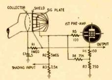
Fig. 4—Detail of first amplifier stage, Fig. 3.
