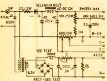
Fig. 4—Battery eliminator for portables.
