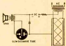
Fig. 2-A gas leak sounds audible alarm.
