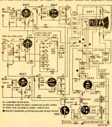
Fig. 1—Ground the junction of the grid and cathode resistors in the lower 65N7 amplifier.
