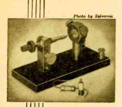
Fig. I-Crystal detectors, the old and new.
